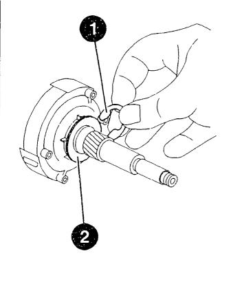
Checking planetary gear train
